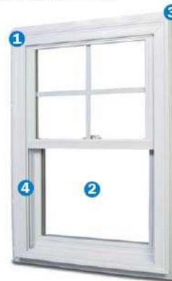
**Easy Installation:** An integral nailing fin gets the Series 3000 into your opening quickly, while a 7/8" 'J' channel siding return allows fast and neat trimming of the exterior siding to the window. Optional wood extension jambs are available for 4-9/16" and 6-9/16" construction, along with a snap-in drywall return channel.
