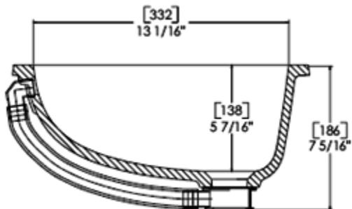
All drain holes are nominally 1 3/4" (45mm) in diameter and accept all standard drain hardware, including waste disposal units. Metric conversions are approximate.
